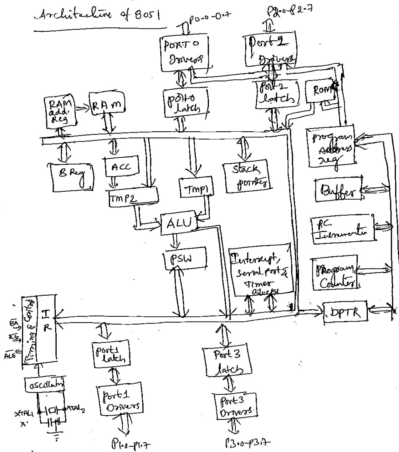
Accumulator (Acc): The Acc (or) it acts as an operand register. This is either be implicit or specified in the instruction. The Acc Register address is allotted in the on-chip Special function register bank.
