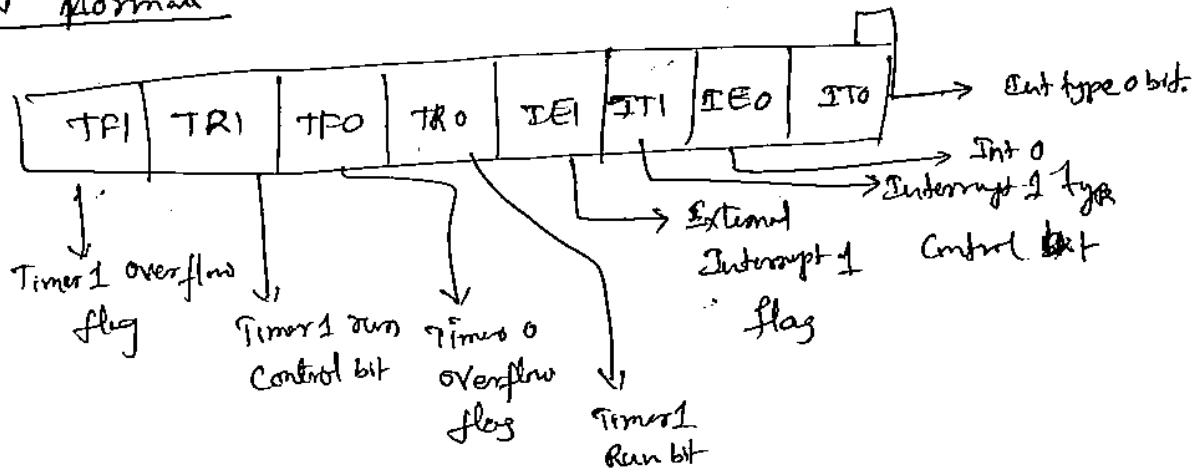
TF1 → this is set by H/w when Timer/Counter 1 overflows & is cleared by H/w as processor vectors to the interrupt service routine.
