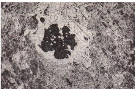
**Microstructure of Malleable Cast Iron**
