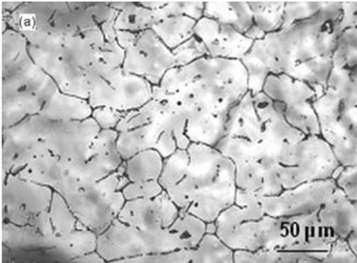
**Optical Microstructure of a 99.5% pure aluminium**
