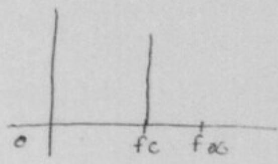
$\Rightarrow$  As  $f_\infty$  will be always greater than cut off frequency, the value of  $m$  will be less than 1.
