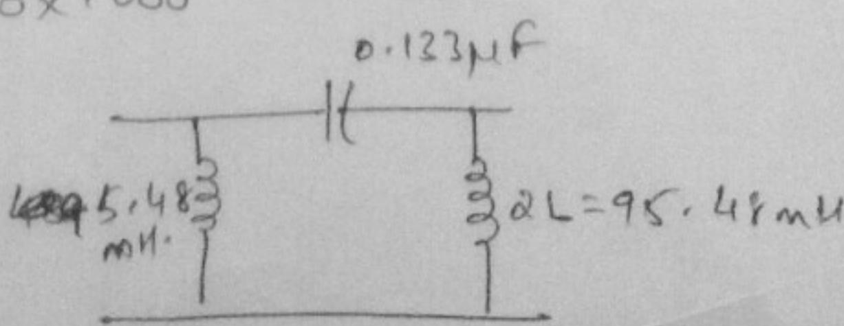
3) Design a m-derived low pass filter having cut-off  $f_2$  of  $1\text{kHz}$ , design the impedance of  $400\Omega$ , and the resonant freq of  $1100\text{Hz}$ .
