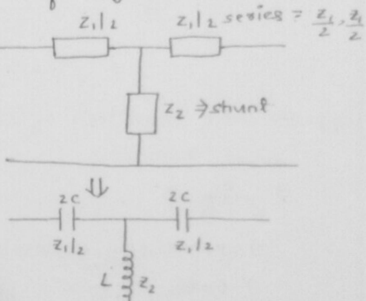
→ The characteristic impedance of symmetrical T-network is
