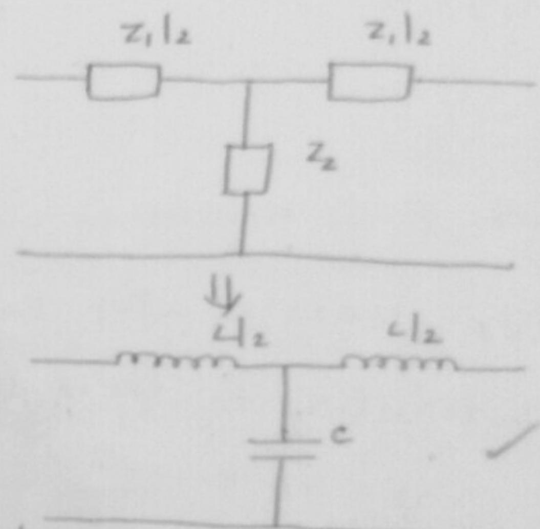
→ The characteristic impedance of symmetrical T-network, is
