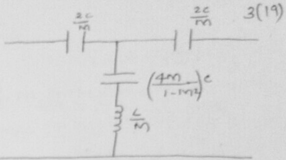
$\rightarrow$  At infinite attenuation frequency, the shunt branch will resonate where the condition is  $x_L = x_C$ .
