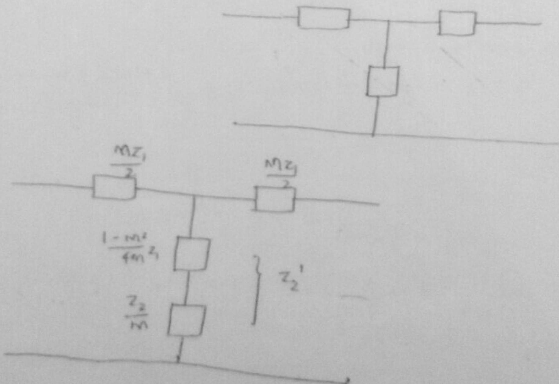
ii) symmetrical  $\pi$ -filter for High pass filter:-
