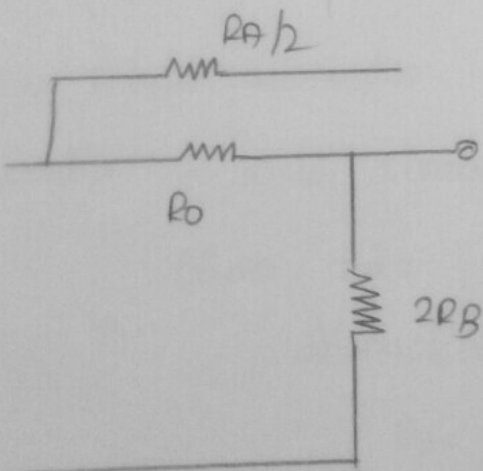
$$R_{OC} = R_0 + 2R_B \quad \text{--- (2)}$$
