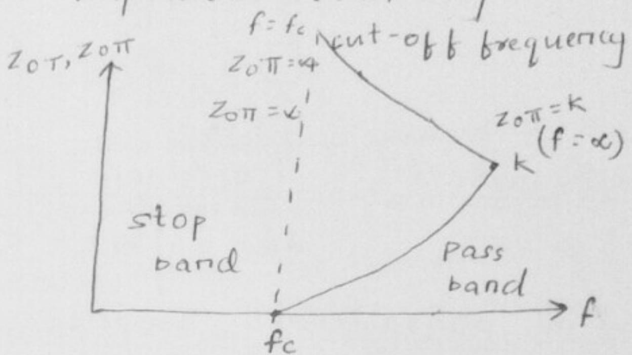
16.11.13 M-derived filters :- As the attenuation in the stop band for a prototype filter is not infinite (or) is not sharp there is a need for us to go for a new filter which will produce sharp attenuation in the stop band. This can be achieved in 2 ways,
