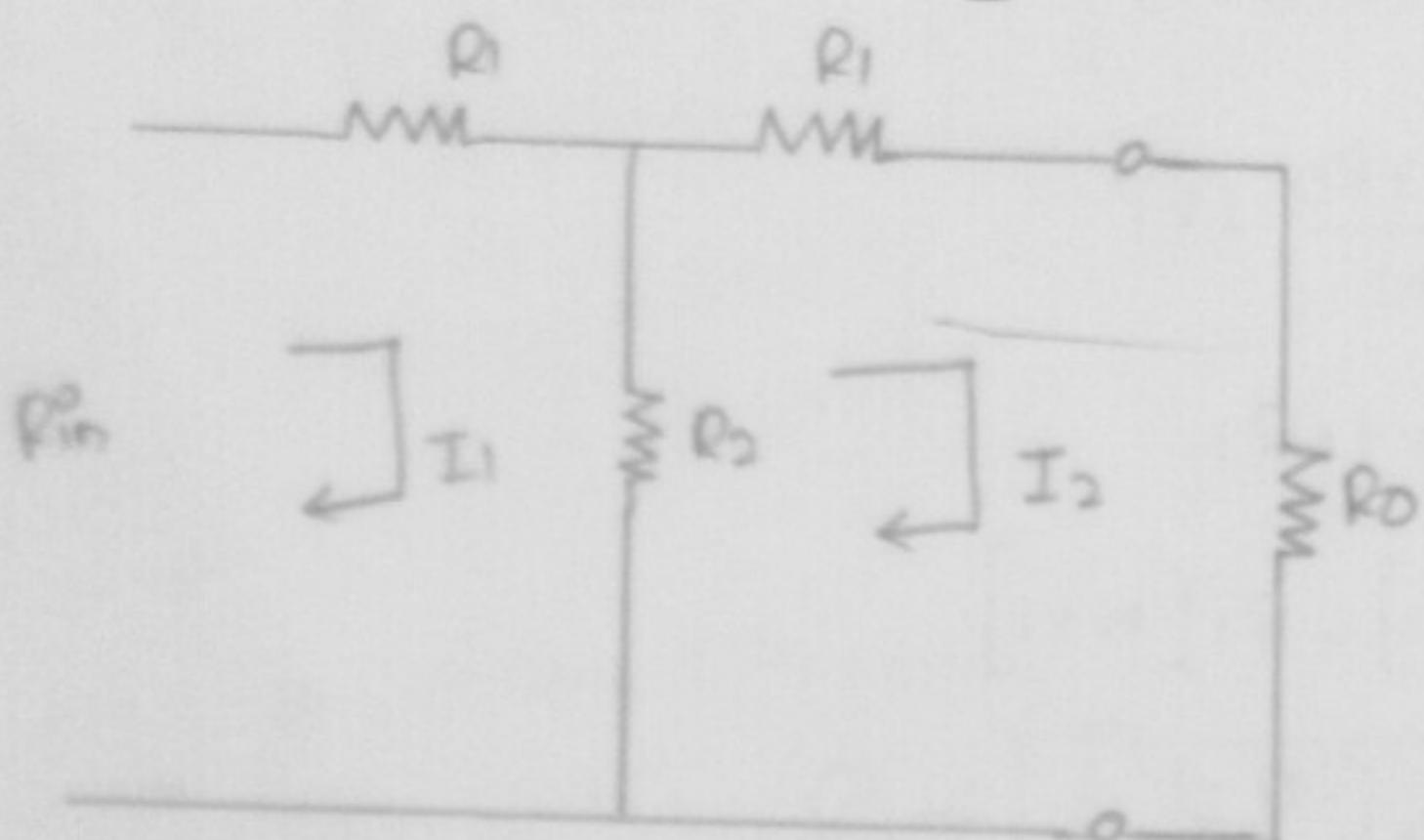
It is an attenuator whose structure look like a T symbol with equal series arm resistance. The symmetrical T attenuator is shown in above fig.
