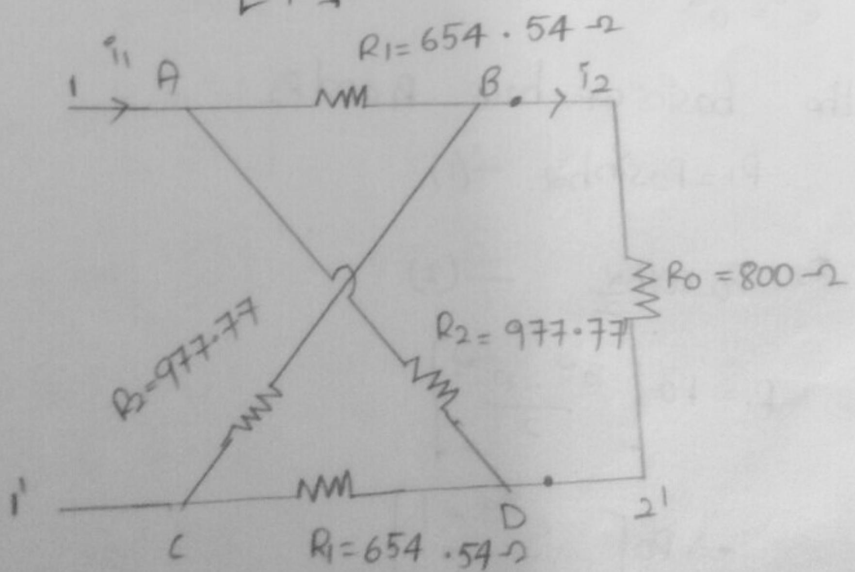
$$\textcircled{1} \quad (R_2 - R_1) - i_2 (2R_0 + R_1 + R_2) = 0$$
