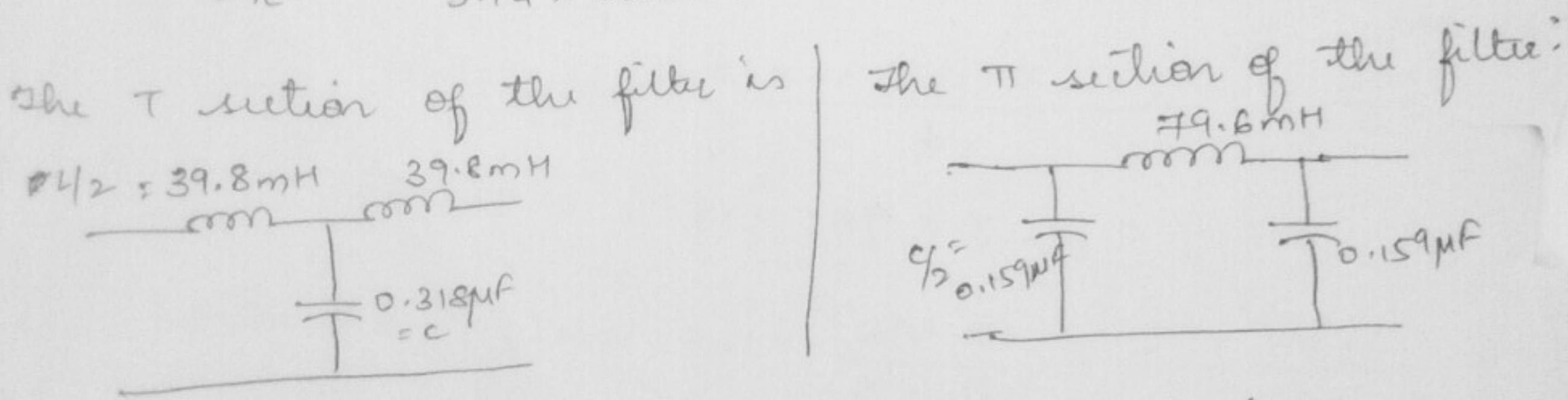
Design a high pass filter having a cut off frequency of  $1\text{kHz}$  with a load resistance of  $600\Omega$ .
