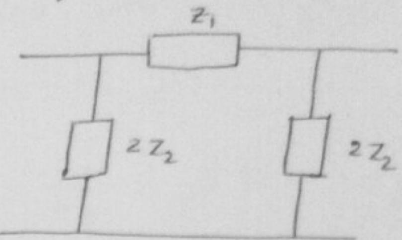
→ The characteristic impedance of symmetrical  $\pi$ -network is,
