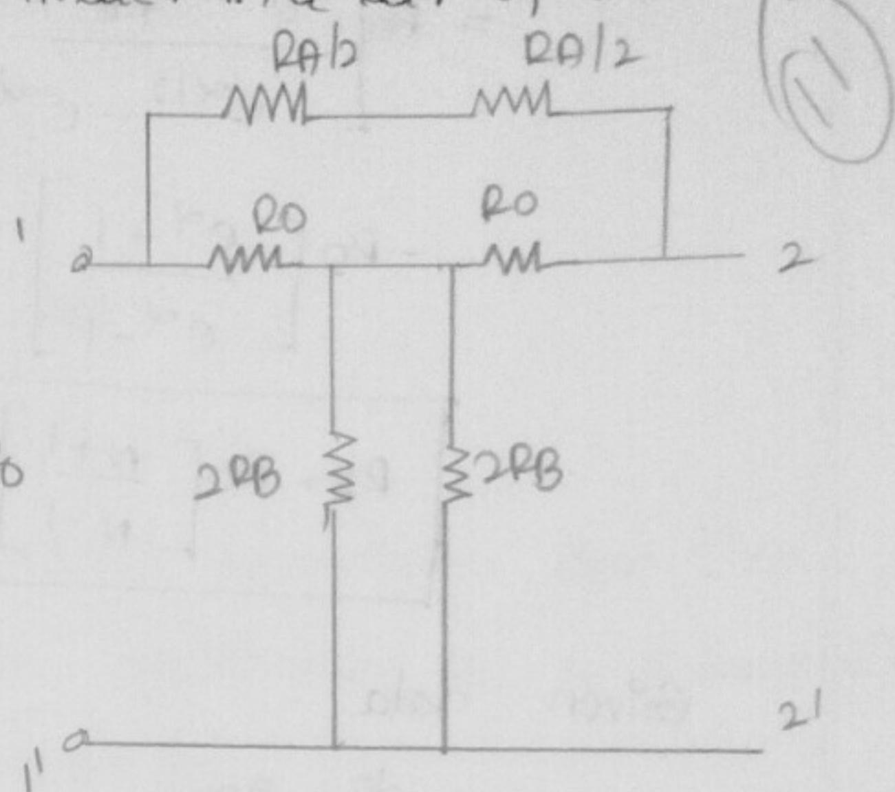
It is similar to the T-attenuator with extra bridge over it. This attenuator is said to be symmetrical when its series arm resistance is equal. The design of the bridged T-symmetrical attenuator will be carried through bisection theorem.
