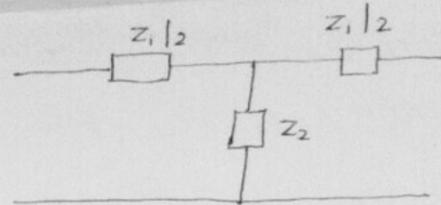
$\Rightarrow$  characteristic Impedance of prototype T-filters :-
