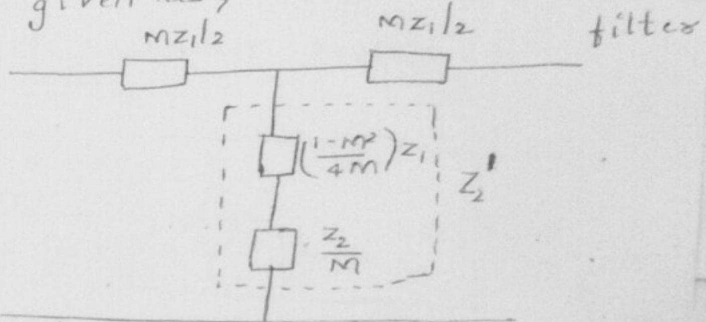
$M$ -derived Low pass filter of T-section:-
