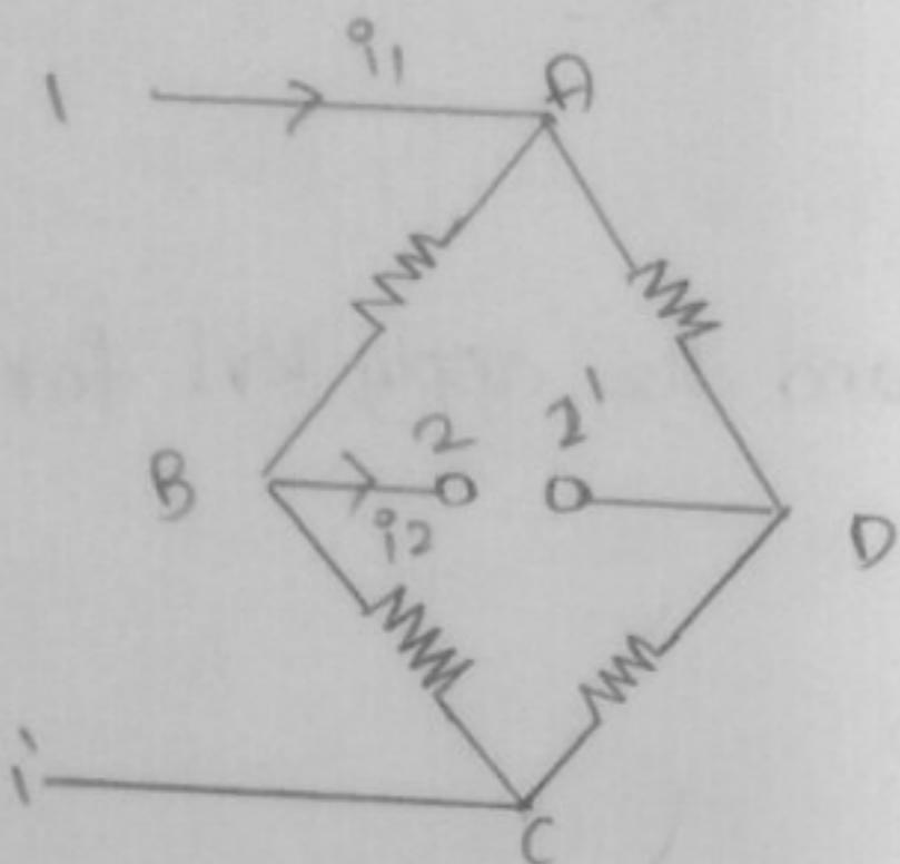
$$R_{oc} = (R_1 + R_2) \parallel R_1 + R_2$$
