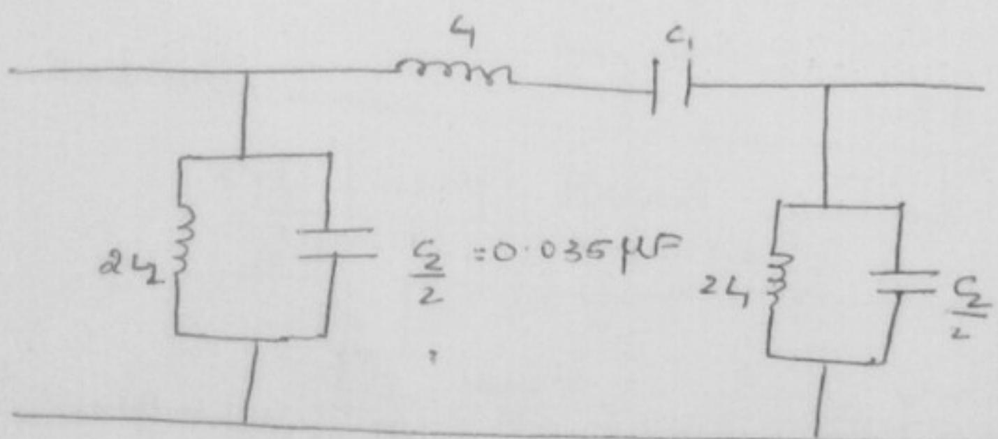
Q:- Design a symmetrical BPF of T & π sections whose cut off frequencies are 3kHz and 5kHz, the nominal impedance is given as  $600\Omega$ .
